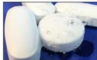
Magnesium chloride tablet (round) rapidly absorbed water from air, damaging it and adjacent pills
